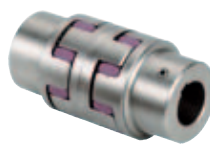
ROTEX® DKM Compensating for extremely big shaft misalignments, Easy assembly Small shaft distance dimension
